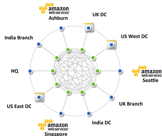
An Aryaka customer's locations, data centers and Amazon instances are meshed to Aryaka's closest POPs to leverage transport of all traffic across one optimized network.
