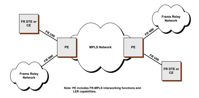
FR-MPLS network interworking connects two frame relay networks and/or devices using an MPLS network. In this architecture, frame relay networks and devices act as CE entities according to the PWE3 architecture. The frame relay service is first provisioned between each frame relay device and the corresponding PE device. A Virtual Connection Label Switched Path (VC LSP) is then set up between the two PEs to complete the frame relay Virtual Connection (VC).
